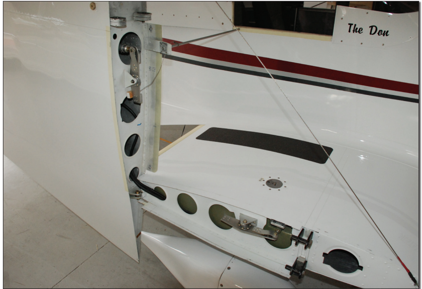
No aileron hookup is required because the center walking beam can always push against its outer counterpart. The inboard wing fuel tank filler is located here.
