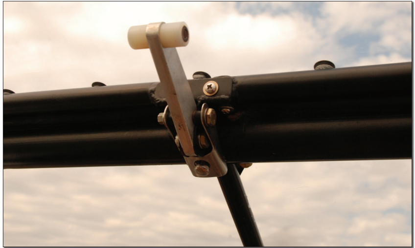
World's best view of a canopy latch: closed, with a turning prop ahead, sky above and the earth far below
