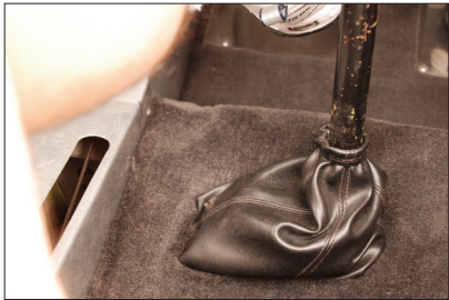
The boot around the controls stick is a nice touch, but makes it a little harder to get in and out. You don't want to step on the mechanism under the boot.
