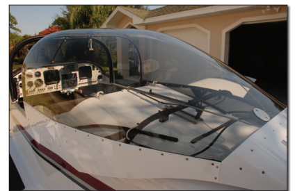
The canopy is from a Thorp T-18, but the windshield is not; it's rounded instead of flat. Note the latch at the top center of the canopy to keep things secure.
