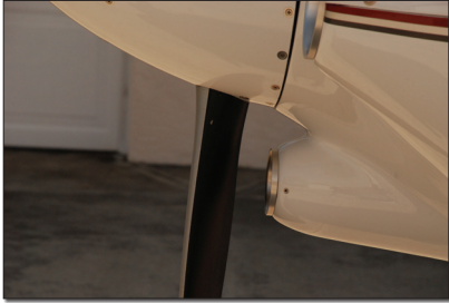
The carburetor air intake undoubtedly gets a boost from being so close to the prop blades. Notice all of the reflections in the fiberglass.
