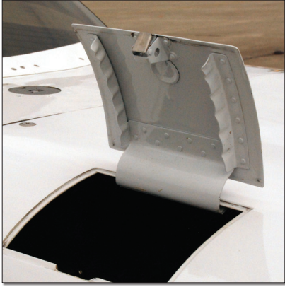
No unsightly piano hinge on this door. And note the nice, even fluting that gives the stiffeners their curved shape.
