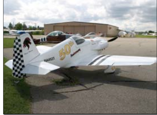
Some 60 years after its inception, the Midget Mustang still has plenty of ramp appeal. The razorback fuselage is frequently replaced by an M1A bubble canopy option for improved visibility.
