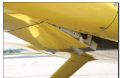
Kinder installed an adjustable cowl flap under his cowl to lower oil temperatures during hot-weather climbs, but says it's only required in extreme conditions.
