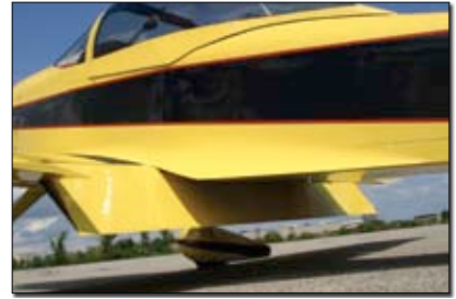
The Mustang II uses a wide manually actuated flap that spans the center section under the fuselage as well as the inner portion of the wing.
