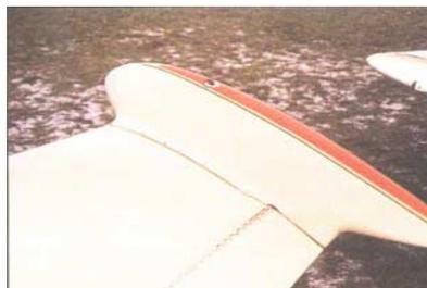
Wingtip tanks have been used to increase the range of the Mustang II.
