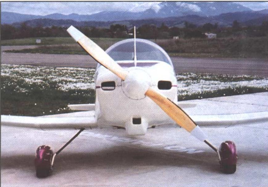
This Lycoming 0-320 powered Bushby Mustang II from Jim Lewis of Walnut Creek, CA, proved to be an excellent performer. Com antenna is forward of the canopy. The propeller was beautifully refinished by Ted Hendrickson following rain damage to the leading edge.
