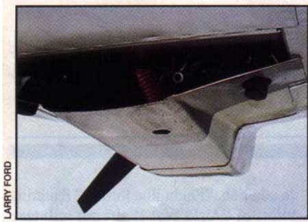
The cowl exit area was reduced by 70% to cut cooling drag.
